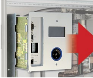
Control elements are easy to remove
