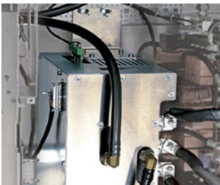
Modules (filter unit and power element) can be released from the front with just a few bolt/plug connections
